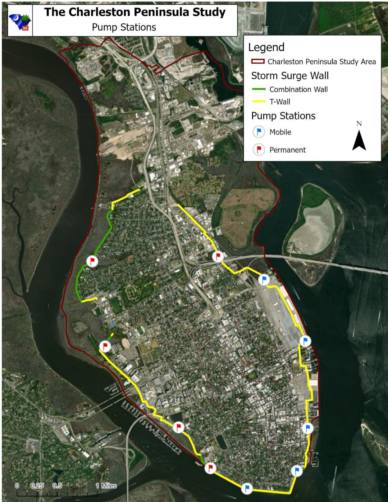
Figure 6-2. Approximate locations of proposed permanent and temporary pump stations.
