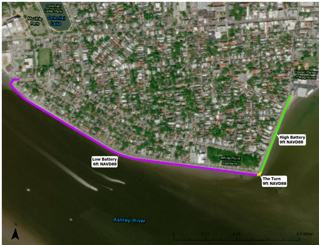
Figure 3-2. The Low Battery Wall is currently being rebuilt and raised by the City of Charleston.
